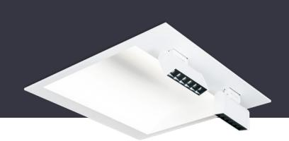
The translucent bent acrylic is purposely chosen as a reflector for indirect lighting. It absorbs and lets small amount of light travel in and out and so it softens the glare of powerful LED light. Aims non-disturbing refine light gradation on the ceiling.
